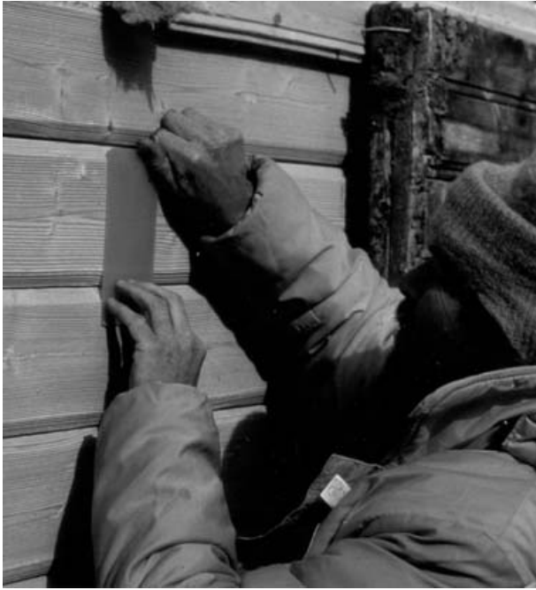
Fig. 5b. Obtaining dental wax cast from north wall boards 'stores hut'. January 1990.
